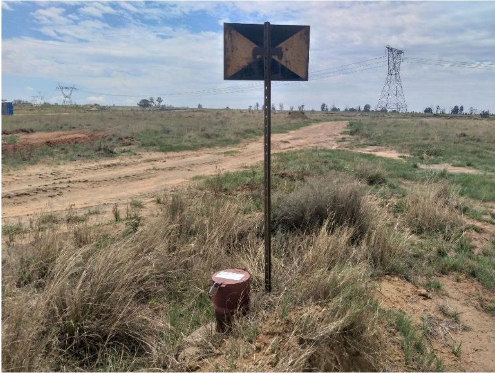
Figure 6: Groundwater monitoring borehole.
