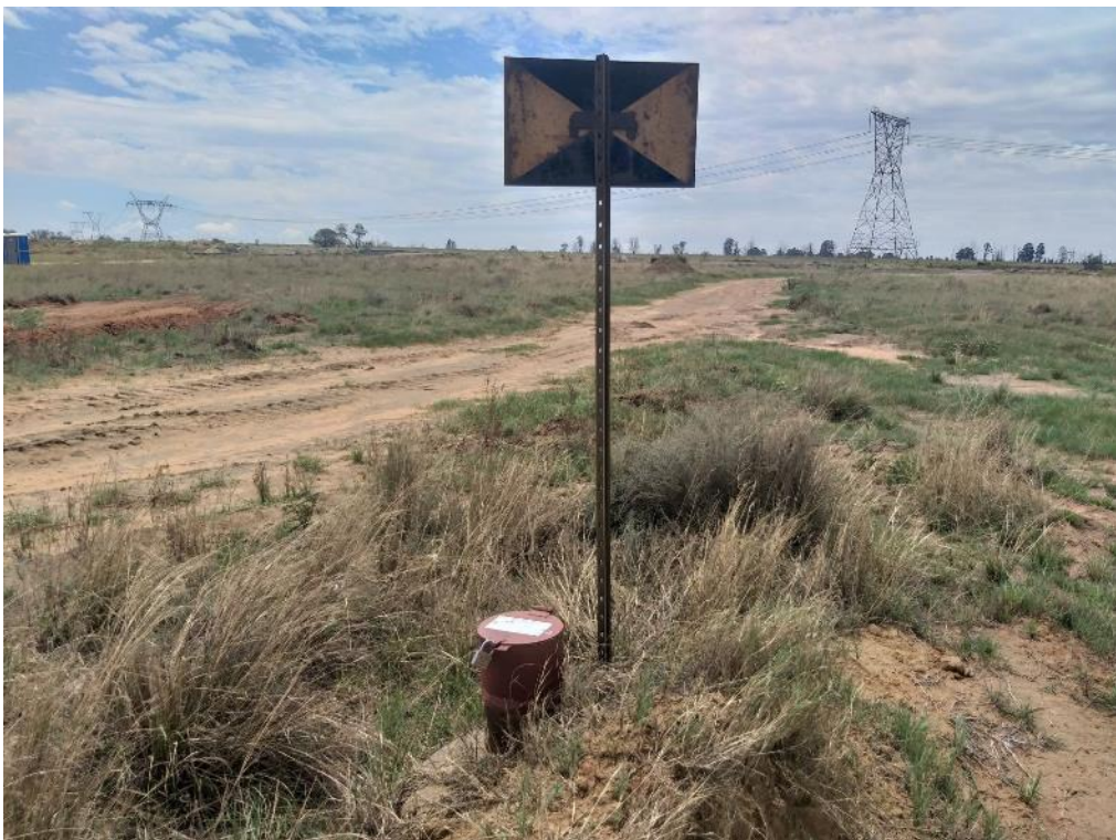
Figure 9: Groundwater monitoring borehole.
