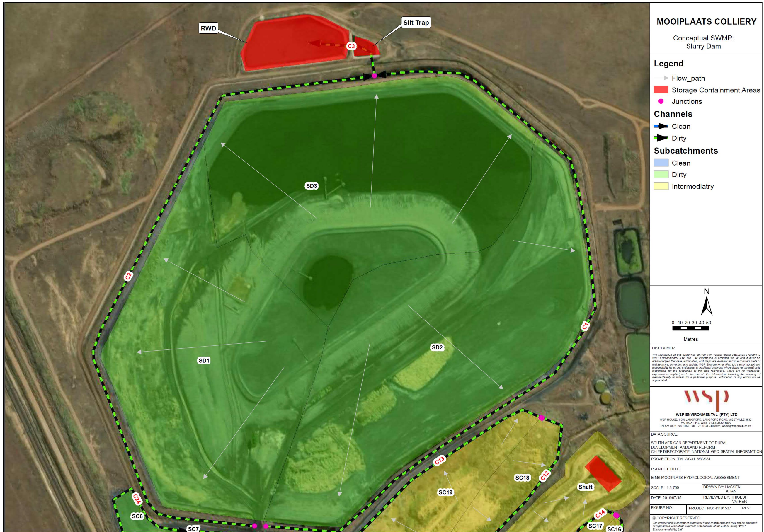
Figure 41: Conceptual SWMP slurry/co-disposal am
