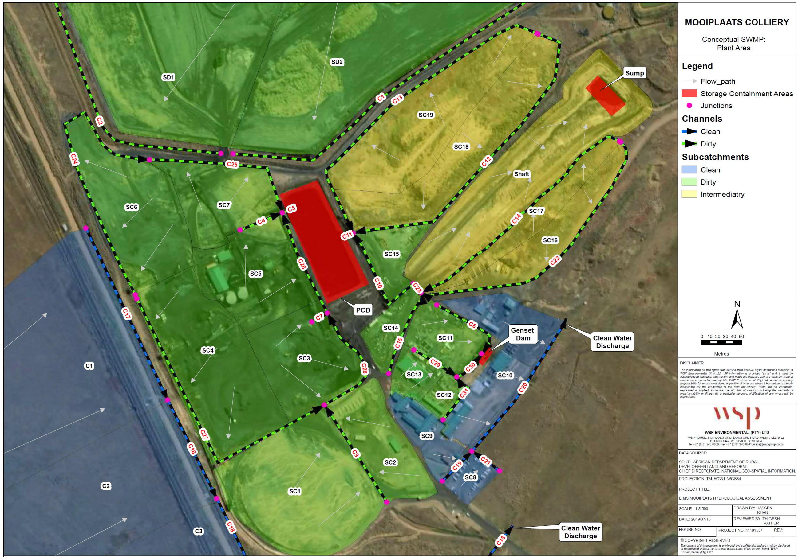
Figure 40: Conceptual SWMP plant area.
