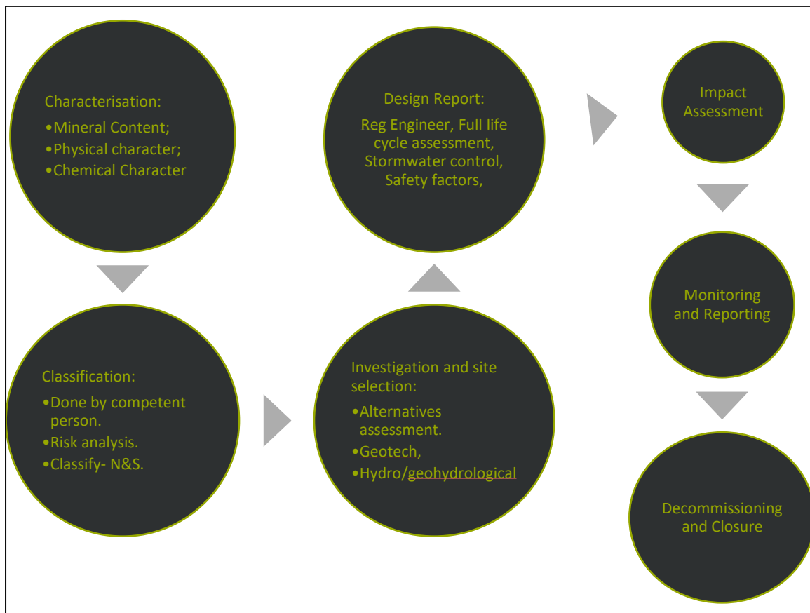
Figure 20: Overview of the planning and management of residue stockpiles and residue deposits regulations
