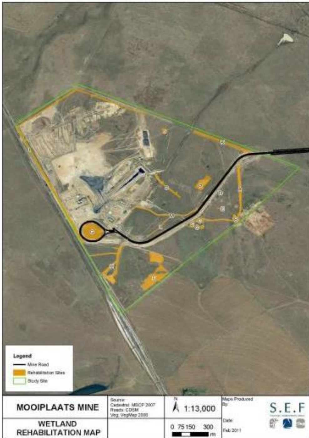
Figure 16: Access roads, stockpiles and general disturbance requiring rehabilitation within wetlands. (Courtesy of the Mining Right EMPr, prepared by Cabanga in 2012.)
