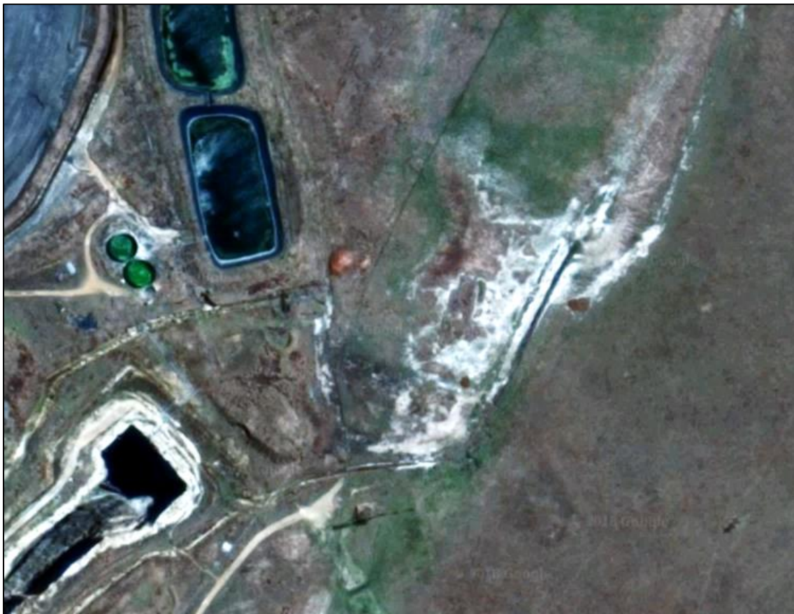
Figure 23: Illustration of likely salts below the Mooiplaats operation, upstream of site MPD (Google Earth Imagery, 2017; 26° 38.566'S 30° 6.115'E)
