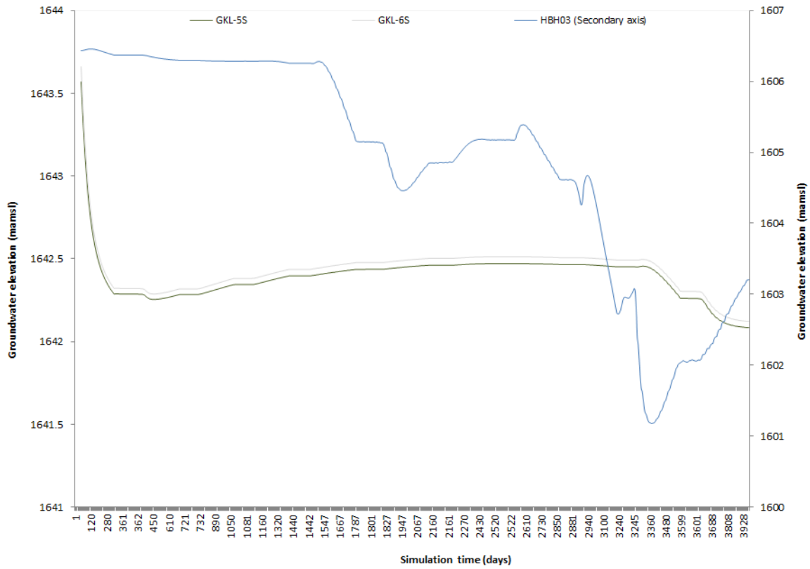
Figure 12-15 Scenario 02a : Curve indicating influence of dewatering on neighbouring borehole water levels.
