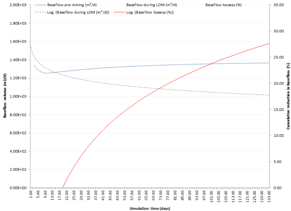
Figure 12-16 Scenario 02a: Baseflow comparison curve: Pre-mining vs underground dewatering.
