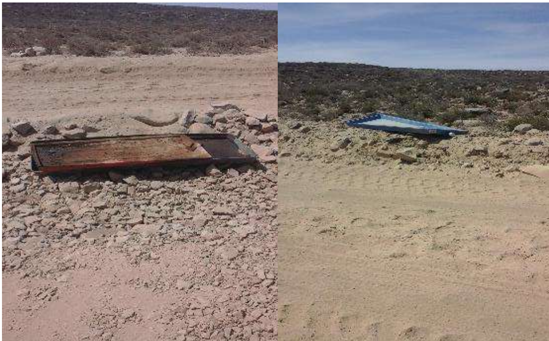
Figure 17: Hydrocarbon contaminated geyser trays used as drip trays on site.
